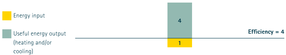
Figure 10 EFFICIENCY OF A HEAT PUMP: THE RATIO BETWEEN USEFUL ENERGY AND ENERGY INPUT
